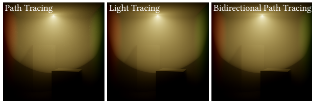
Fig. 12. We render the same scene with different rendering algorithms and obtain identical results regardless of transport direction. This supports the fact that our method is reciprocal.
