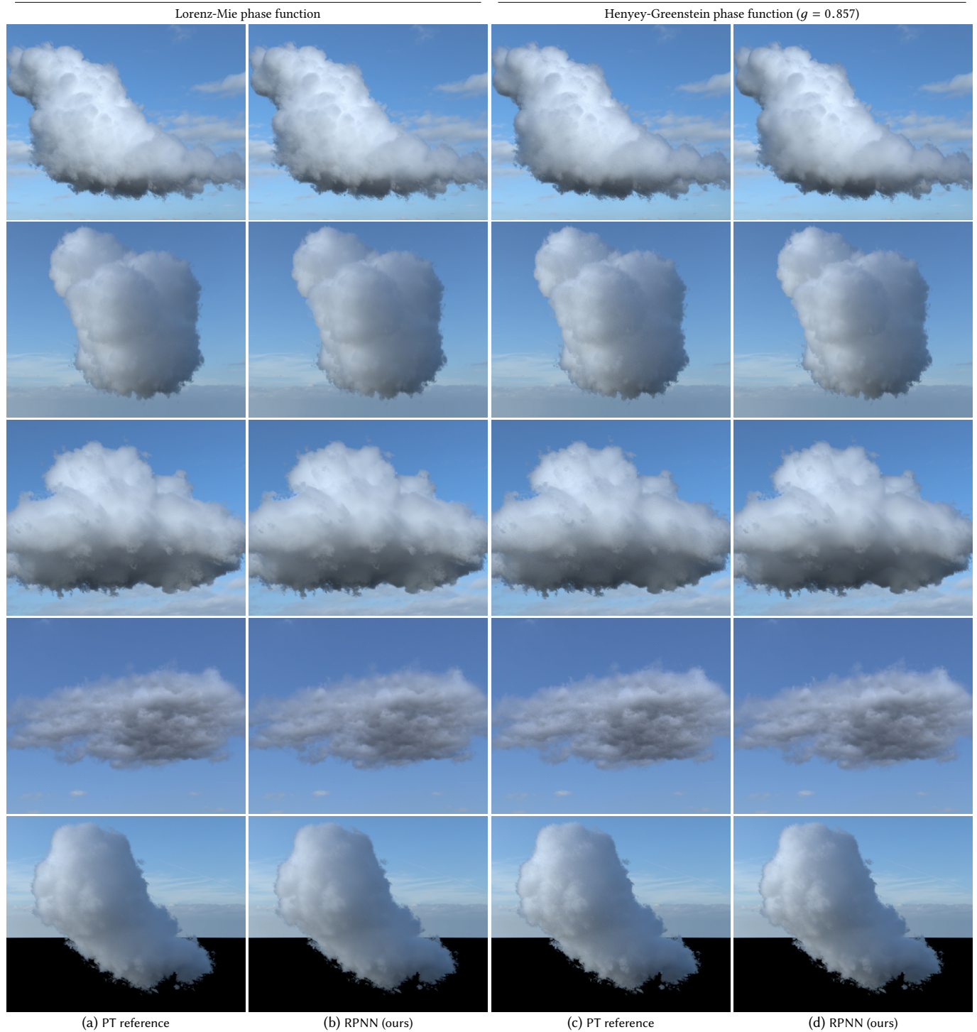
Fig. 5. Comparison of a path-traced reference and our radiance-predicting neural network (PRNN) on side-lit clouds illuminated by an environment map.
