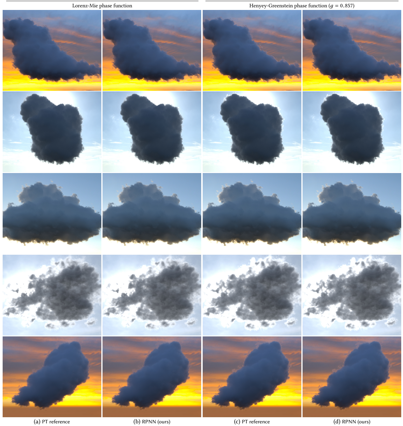
Fig. 7. Comparison of a path-traced reference and our radiance-predicting neural network (PRNN) on back-lit clouds illuminated by an environment map.
